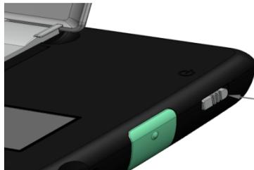
Slide the spring-loaded power switch toward rear, then release
